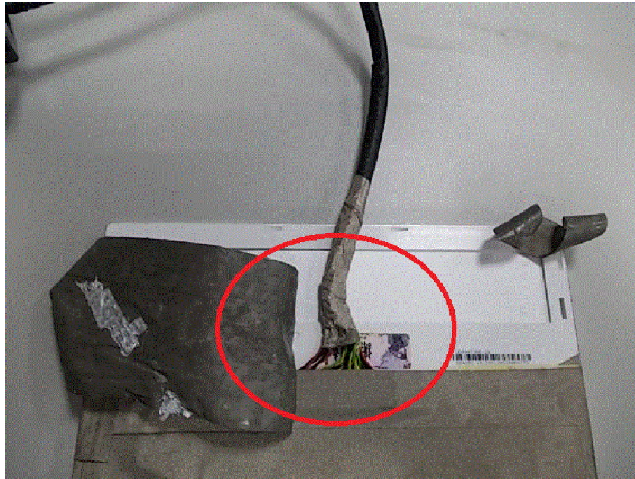
LCD CABLE PANEL 端 SHIELDING 示意圖 1
